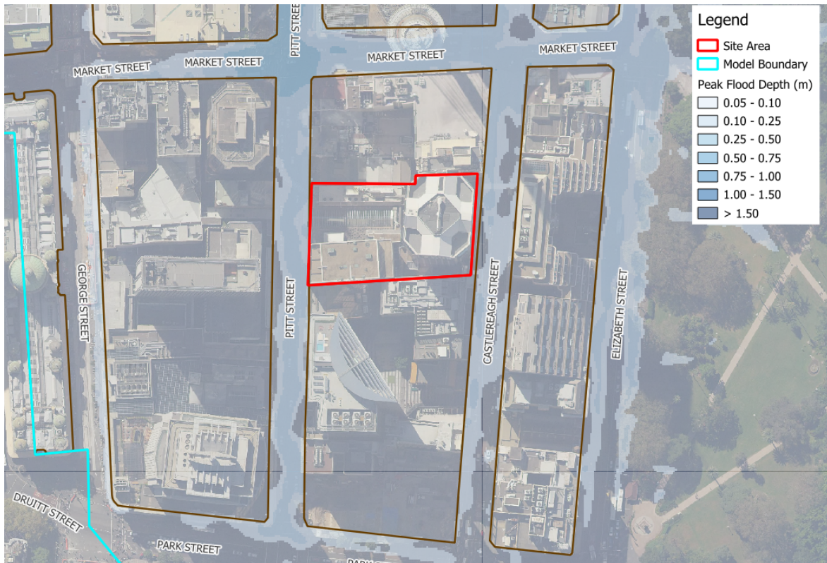
Figure 9: Peak Flood Depths – 1% AEP Event (100 Year ARI) Results extracted from supplied TUFLOW model (note flood depths clipped where < 0.05 m)
